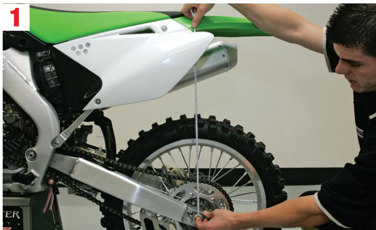
**1.** Using the tape measure provided, measure the unloaded dimension when your bike is supported by a bike stand and the rear wheel is off the ground. Measure the distance from the rear axle up to a fixed point, like the fender and side panel junction, in line with the arc of the axle. You can also put a mark on the fender, which lines up with an even number to make it a little easier to calculate. Write down as Dimension A (Unloaded Example: 605 mm).
