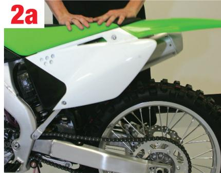
**2a.** The second measurement is taken with the bike on the ground. But first, push down on the seat and slowly let it rise up to its final resting position.
