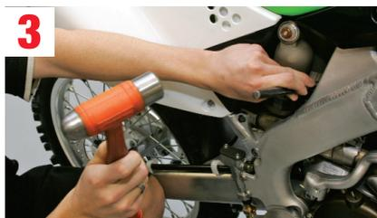
**3.** To change the sag, use a long punch and a large hammer to loosen the spring locking nut on the shock.
