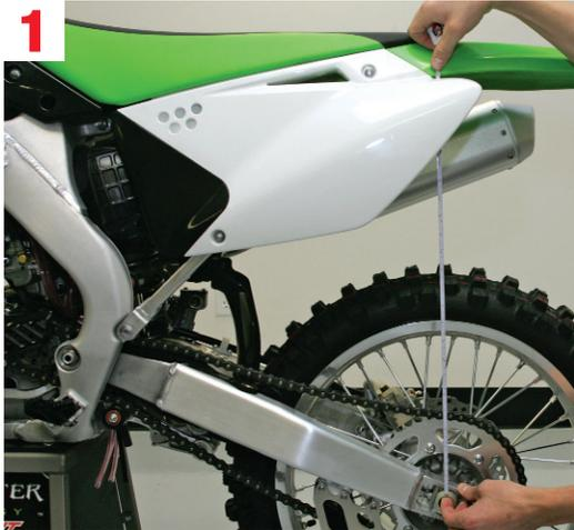
**1.** The first measurement is taken, as earlier, with the bike on a stand, and the rear wheel hanging freely. Measure the distance between the rear axle and the same point used to measure the race sag. This will determine Dimension A (Static Sag Example: 605 mm).
