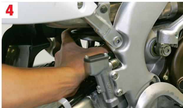
**4.** Then, turn the spring with your hand to adjust the rear spring preload. Make sure that when you're turning the spring, the preload nut is also turning. There may be times where you will need to push on the preload nut with the punch while you're turning the spring.
